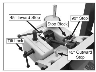
Figure 19. Tilt lock and stop block locations.
